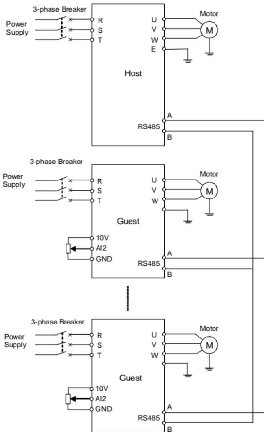
Fig9-4 Basic wiring
