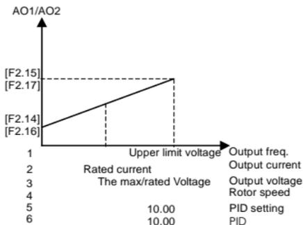
Fig.6-8 output of analog terminals
