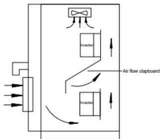
Fig2-1-B Multi-inverter Installation
