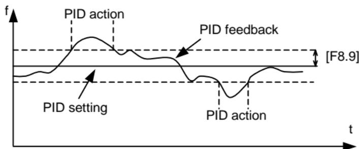
Fig.6-23 PID Control allowable deviation limit
