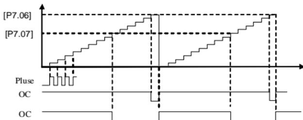
Fig.6-17 Internal counter function
