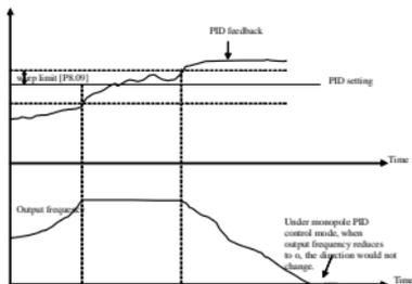
Fig 6-20 Monopole PID control mode
