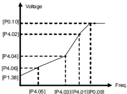
Fig.6-14 V/Fuser-defined curve
