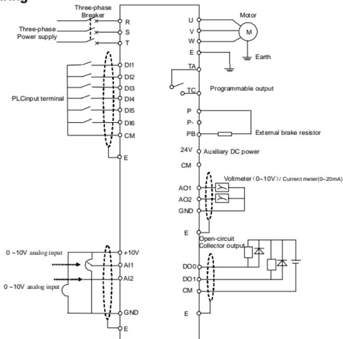
Fig.3-3 V600 series of inverter basic wiring
