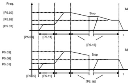
Fig.6-16 PLC recover running after restart
