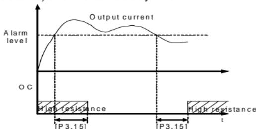
Fig.6-12 Over-load alarm
