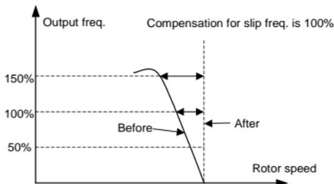
Fig.6-6 Compensate for slip freq.
