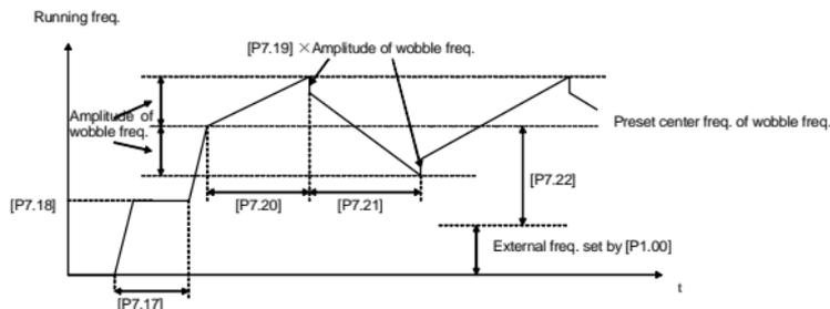
Fig.6-19 Running process of wobble freq.
