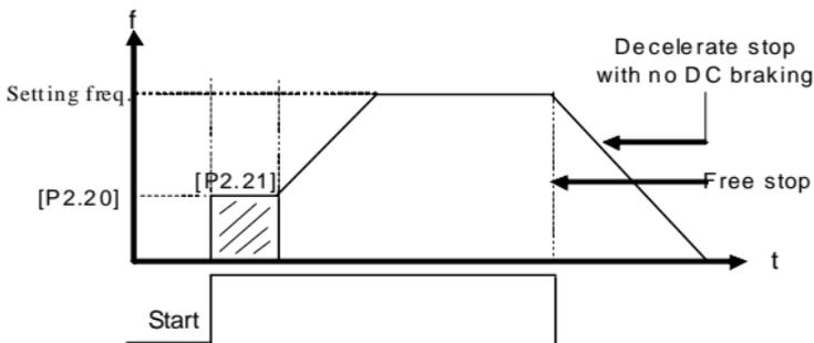
Fig6-1 Start and stop freq. output curve
