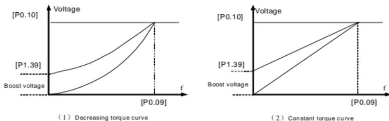
Fig.6-5 Torque boost
