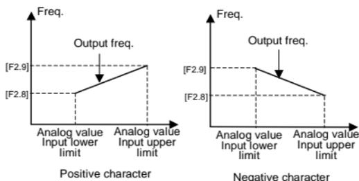
Fig.6-7 corresponding relation between analog input and setting freq.
