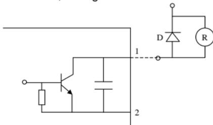
Fig.6-9 Inner wiring diagram of output terminals
