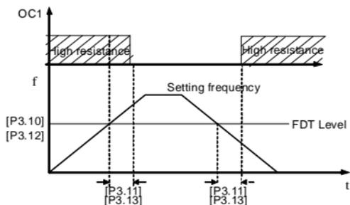
Fig. 6-11 Freq. level detection signal (FDT)
