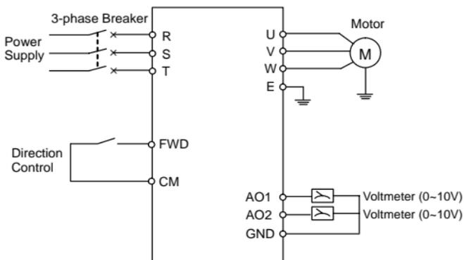
Fig9-1 Basic wiring
