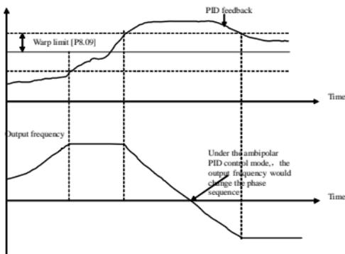
Fig 6-21 Ambipolar PID control mode
