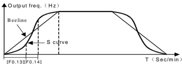
Fig.6-0 Acc/Dec curve
